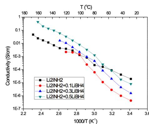
By increasing ratio of  $\text{LiBH}_4$ , the conductivity of the system increases.
