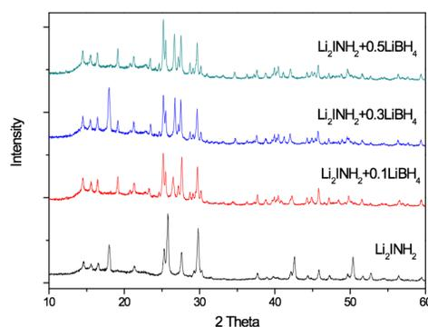
Similar XRD patterns were obtained by changing order of reaction in the ternary system in mechanical reaction. It suggests to the occurrence of a new single phase. So in order to elucidate this, evolution of the phase has been studied.
